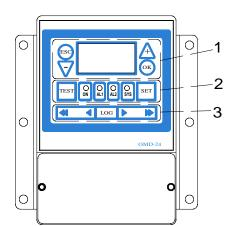
There are 3 groups of push buttons to control the functions of the display. Navigation buttons are in group 1. Functional buttons are group 2. Group 3 is for data logger operation.
