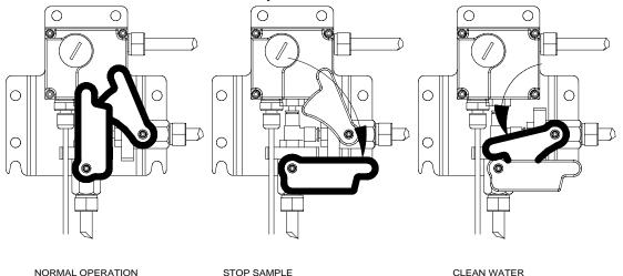
operate the handles. The OMD-24 will only allow overboard discharge in Normal Operation setting of both valve handles.
